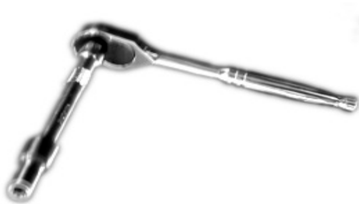
Standard 3/8 th inch ratchet drive with 6" extension and star tuning tip
